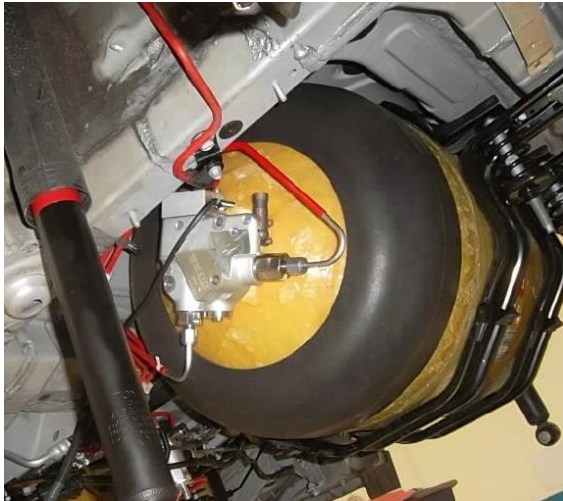
Figure 5 Hydrogen storage cylinder and integrated valve –attached to cylinder in vehicle (left) and schematic of the integrated valve (right) (Mattelaer, 2019)
