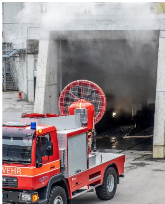
Figure 7. Ventilator in front of IFA railway tunnel
