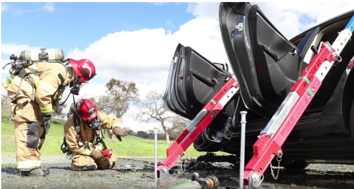
Figure 3 Special pillars for providing access to the batteries in the bottom of an electrical vehicle (TESLA M3)
