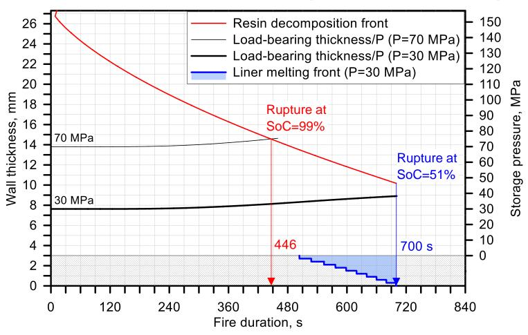
The decrease of tank's SoC to 51% for such tank will result in hydrogen leak and exclude tank rupture.
