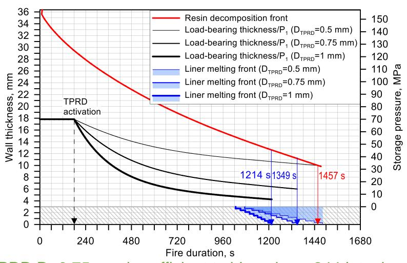
TPRD D=0.75 mm is sufficient to blow-down 244 L tank in a fire of HRR/A=1 MW/m<sup>2</sup>
