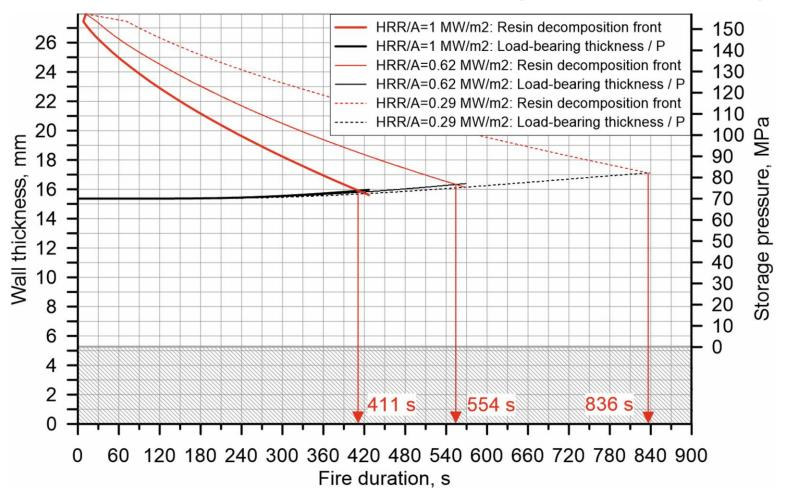
The increase in fire intensity (HRR/A) significantly increases the rate of resin decomposition and thus reduces the time to rupture (FRR)
