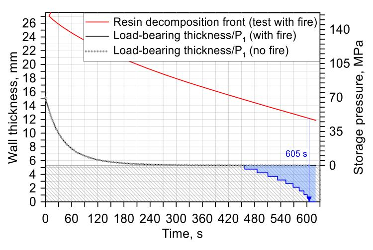
Storage pressure/wall load-bearing thickness
