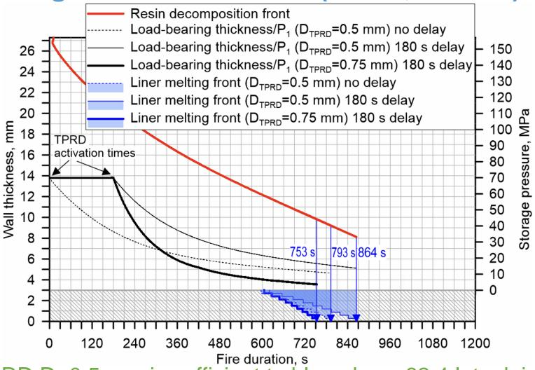
TPRD D=0.5 mm is sufficient to blow-down 62.4 L tank in a fire of HRR/A=1 MW/m<sup>2</sup>
