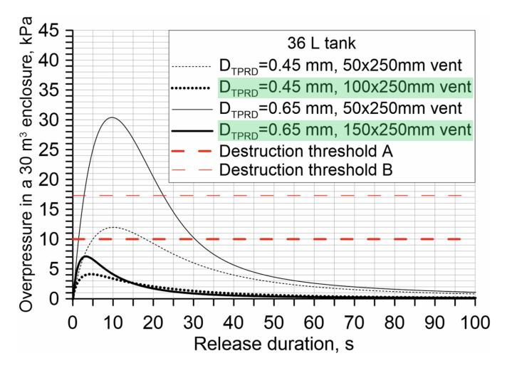
Destruction threshold A: P=10 kPa, threshold B: P=17.3 kPa
