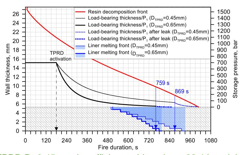
TPRD D=0.45 mm is sufficient to blow-down 62.4 L tank in a fire of HRR/A=1 MW/m<sup>2</sup>
