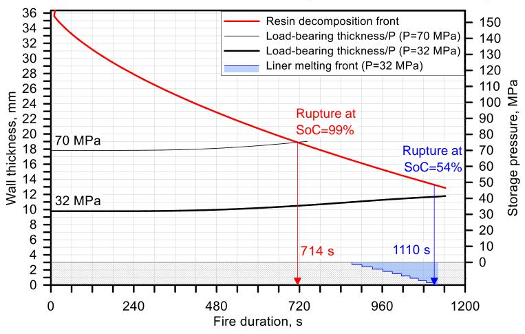
The decrease of tank's SoC to 54% for such tank will result in hydrogen leak and exclude tank rupture.
