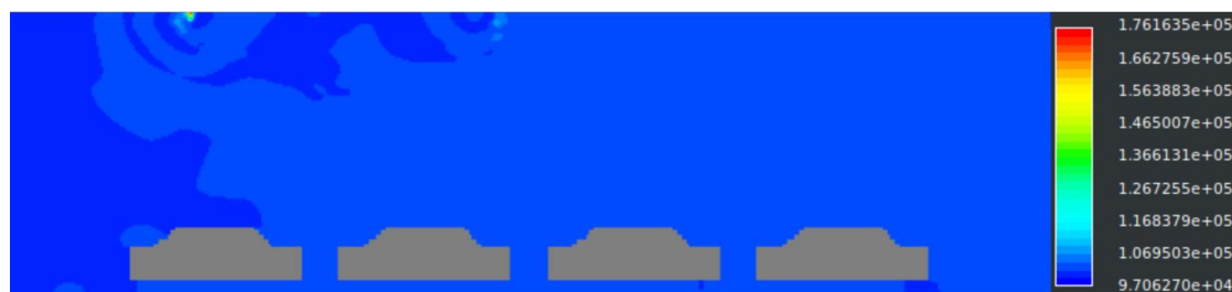
Figure 49. Pressure contour plot at 5.275s for cases without ventilation.
