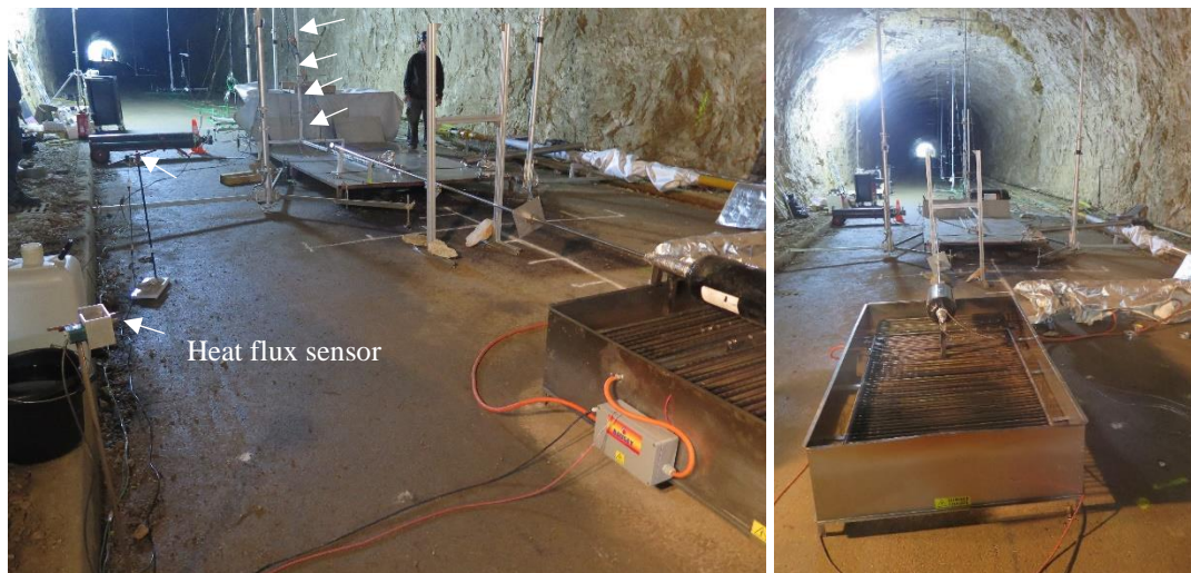
Figure 157. Location of the radiative heat flux sensors.
