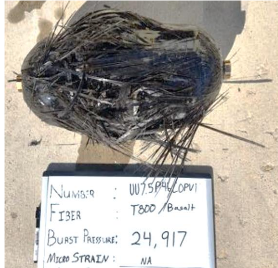
Figure 148. Example of achievement of the burst pressure for prototype No 1: P_{burst}=24,917 \text{ psi}=1718 \text{ bar} , giving the burst pressure ratio 2.45.
