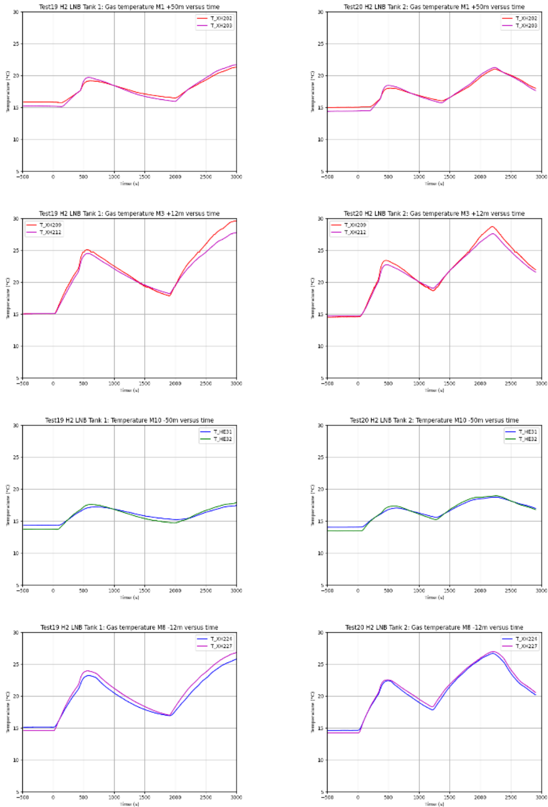
Figure 164. Measured gas temperature close to the top of the tunnel at different distances along the tunnel axis.
