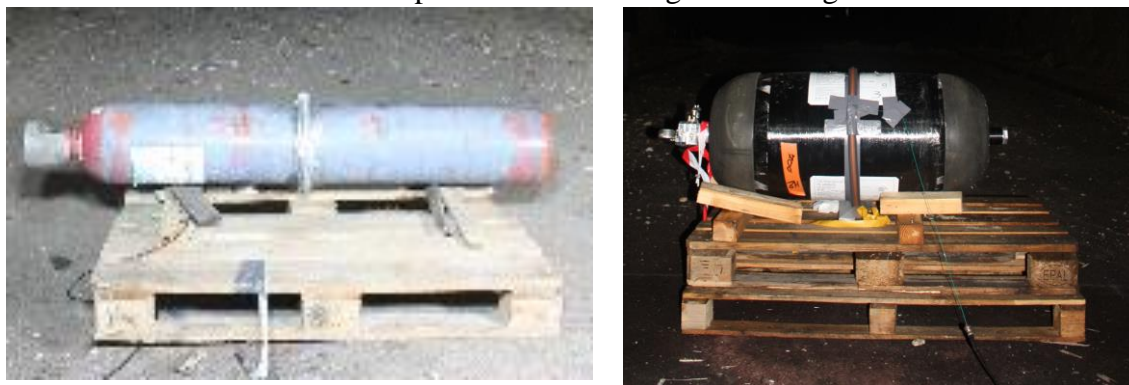
Figure 113 : Tanks used for explosion experiments: TYPE II (left) and TYPE IV (right). The detonation belt is attached to each of the tanks.
