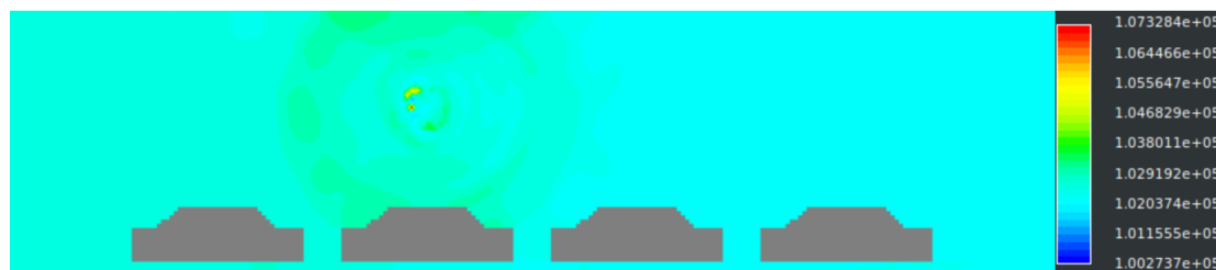
Figure 48. Pressure contour plot at 5.216s for cases with ventilation.
