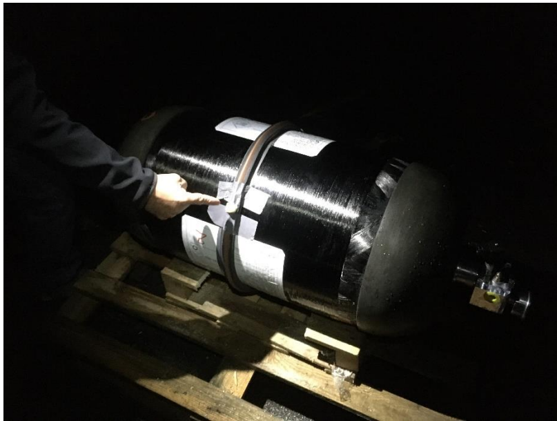
Figure 96. Example of tank equipped with a detonation belt.
