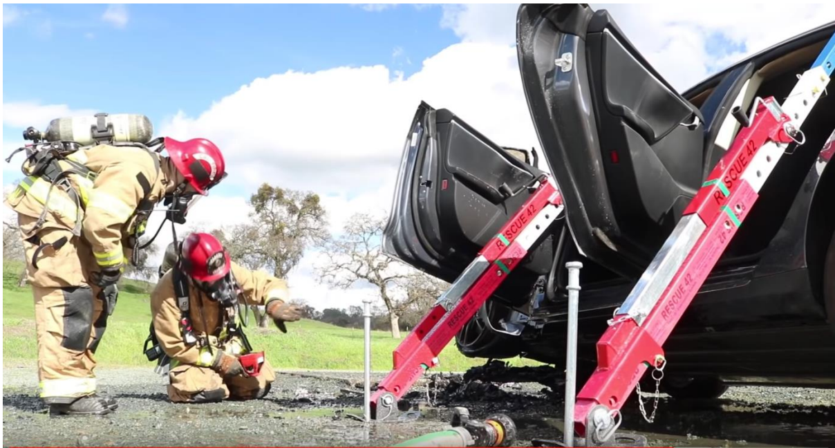
Figure 10. Special pillars for providing access to the batteries in the bottom of an electrical vehicle (TESLA M3).
